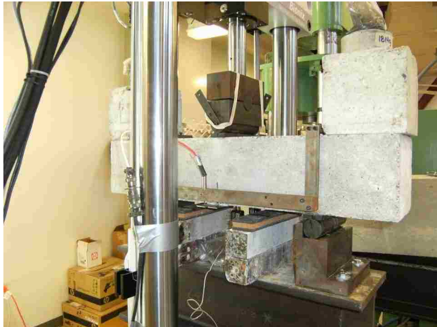
Figure 3.15 – Test setup with counterweights
