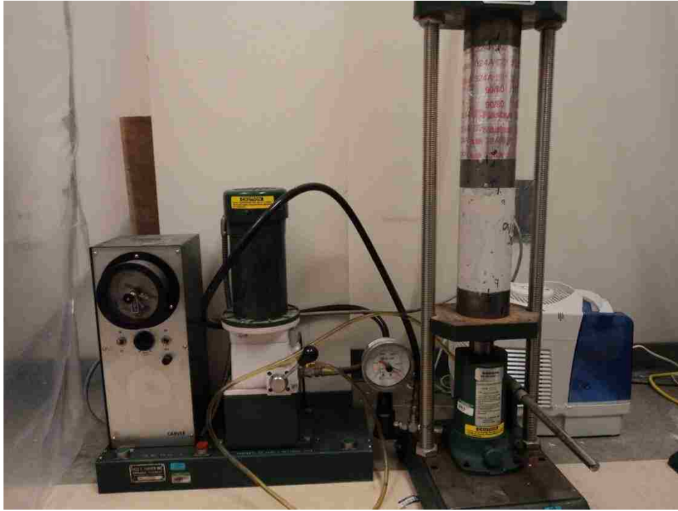
Figure 3.10 – Creep test in progress utilizing creep frame
