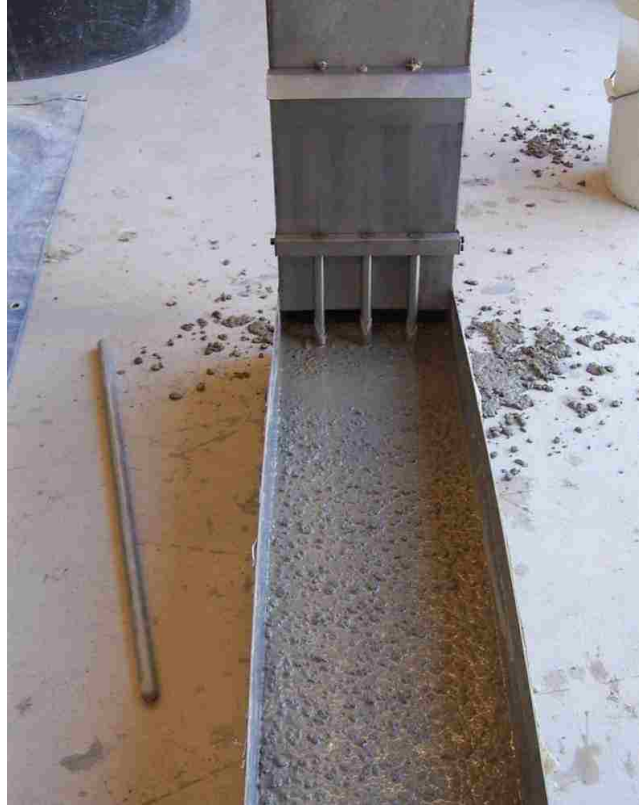
Figure 3.7 – L-Box test to determine SCC passing ability
