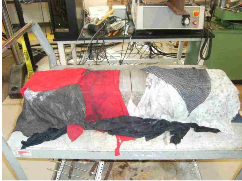
Figure 3.14 - Transporting beam to not allow drying
